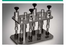
Fixture for mounting specimens to glass slides for thin-sectioning, provides a uniform thickness of bonding material between the specimen and the glass slide, spring activated loading system with capacity upto 8 specimens, easily plcable on hot plate
