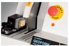
GEOFORM is a universal product that can be used for precision sectioning, re-sectioning and grinding operations
