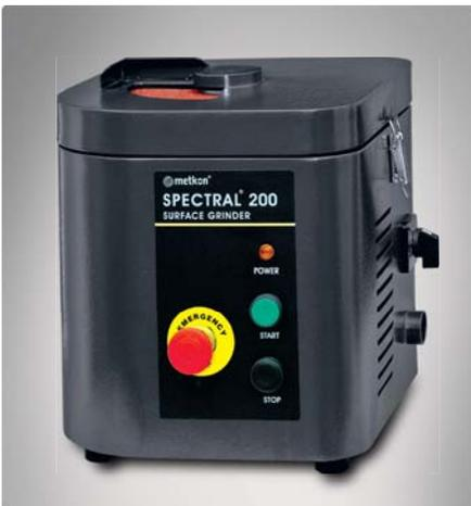
SPECTRAL 200 is a table-top portable surface grinder for the preparation of steel samples for spectroscopy. Its compact design with vibration free operation makes it a practice instrument to work with. Low noise and dust generation levels as well as standard outlet for dust exhauster are additional advantages.
