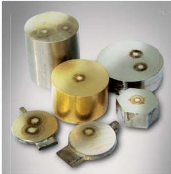
Sample preparation of metals and materials have become more and more important because of the rapid development and improvement of both software as well as OES and XRF-devices during the past few years that shifts the detection limit for trace analyses. It is crucial to have the sample properly prepared. The sample needs to be both representative, homogeneous and with an even surface in order to eliminate factors that can influence the results.
